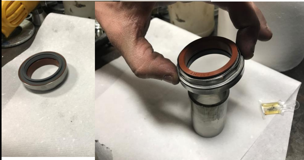
Illustration 12: Seal Orientation on Sleeve
