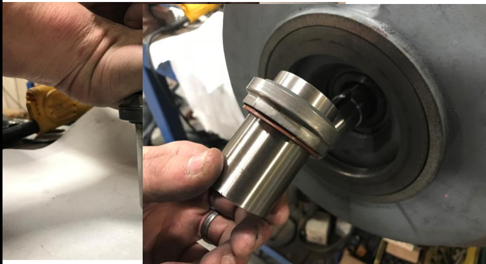
Illustration 14: Hand-Spaced Seal on Sleeve
