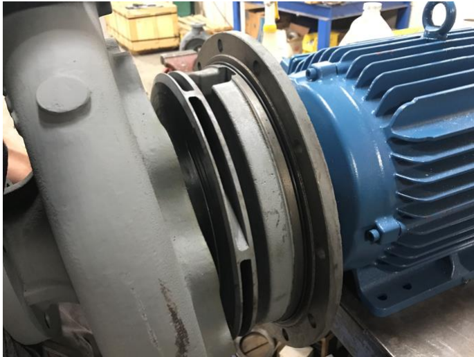
Illustration 21: Installing the Pump Case
