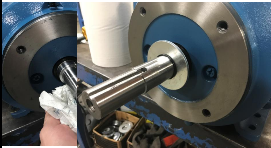
Illustration 2: Cleaning the Motor Shaft
