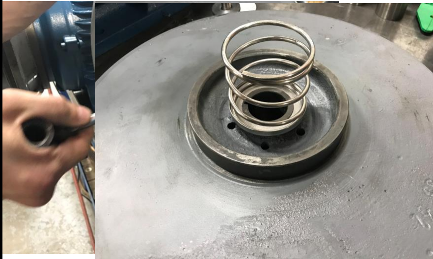
Illustration 10: Checking Seal Spring Fit on Impeller
