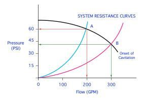
A manufacturer's pump curve also gives information on efficiency, actual horsepower consumed, suction head pressure requirements, and the effect of changing impeller size or speed of rotation. The simplified curves above are for illustration only.
