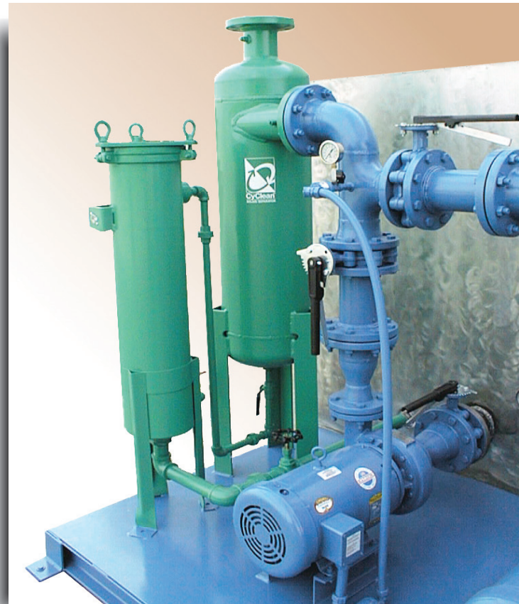
CyClean™ CYB-400 4" centrifugal separator with 2" bag filter for full stream cleaning of 350 GPM of cooling tower process water. Features zero water discharge and easy solids removal without interrupting system operation.
