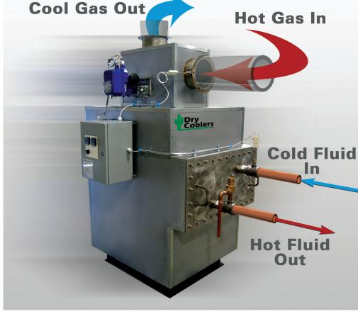
Designed specifically for high temperature industrial gas streams, HRU heat transfer packages incorporate state of the art features optimized by 3-D solid modelling for the ultimate in reliability and maintainability.
