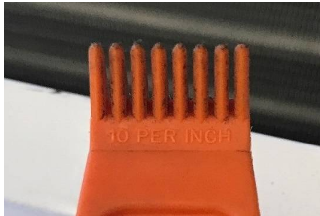
Illustration 4: Fin Comb with 10 FPI
